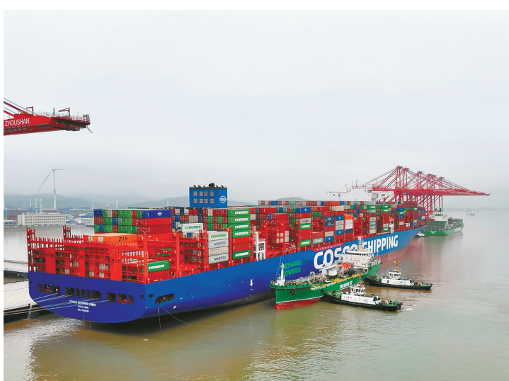
Ship-to-ship green methanol bunkering operation at the Meishan port area of Ningbo Zhoushan Port. [Photo by Lin Yuchen]
